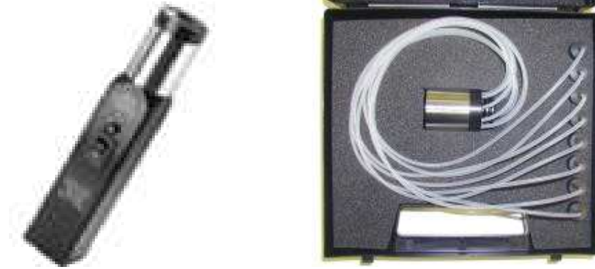
Figure A.8: G.R.A.S Pistonphone type 42AA and Octopus adapter type RA0025.
