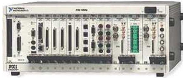
Figure A.5: A representative photograph of an 18 slot PXI-1006 chassis.
