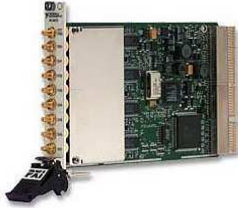
Figure A.6: An 8-channel PXI NI-4472 Dynamic Signal Acquisition module.
