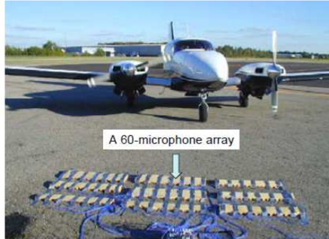
Figure 4.11: Test setup for a twin propeller aircraft.
