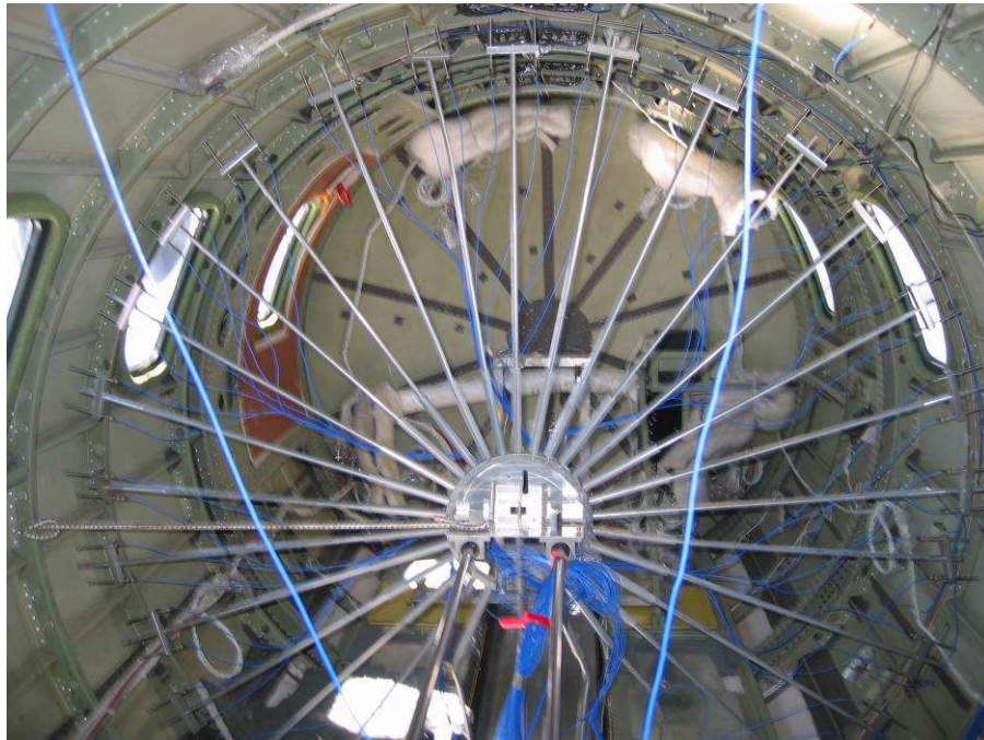
Figure 5.4: 60 microphone conformal array with telescoping arms for circumferential measurement.
