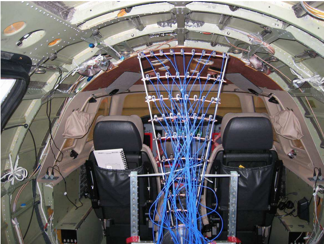
Figure 5.6: Picture of planar array used to measure the closing surface.
