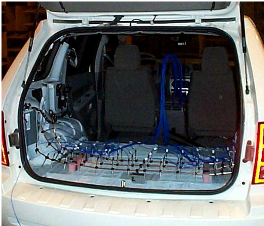
Figure 2.9: A typical partially enclosed interior test setup.
