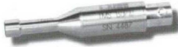
Figure A.3: The ICP ® Microphone Cartridge Model No. TMS130C10 and Pre-Amplifier Model No. TMS130P10.
