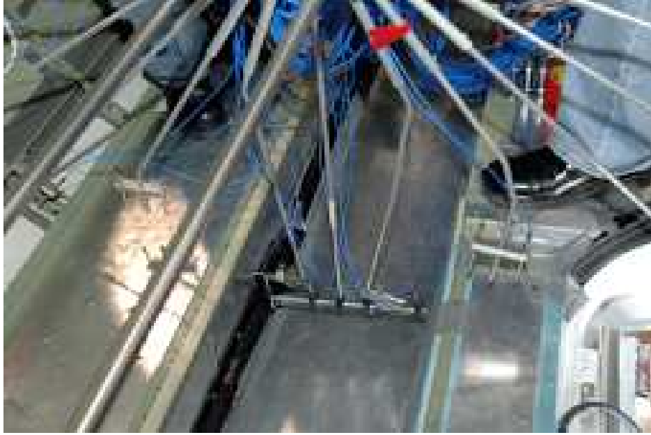
Figure 5.5: Part of the conformal array used for measuring over the floor panel.
