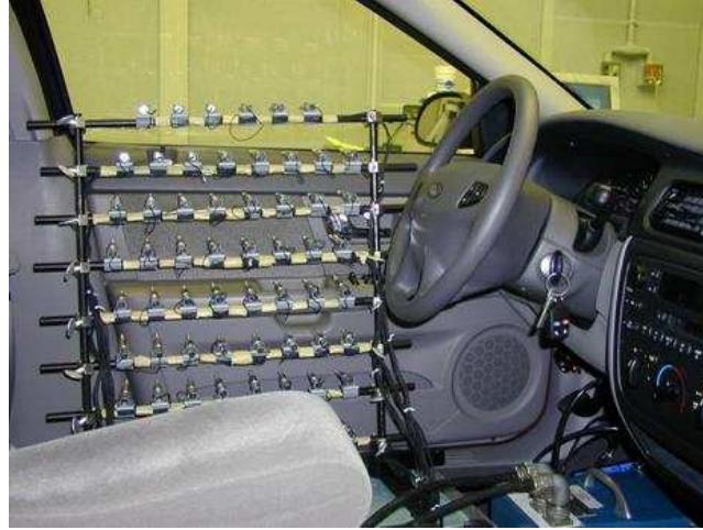
Figure 2.8: A typical completely enclosed interior test setup.
