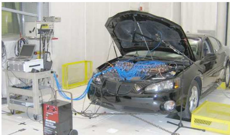
Figure 2.7: A typical bounded or non-free field exterior test setup.
