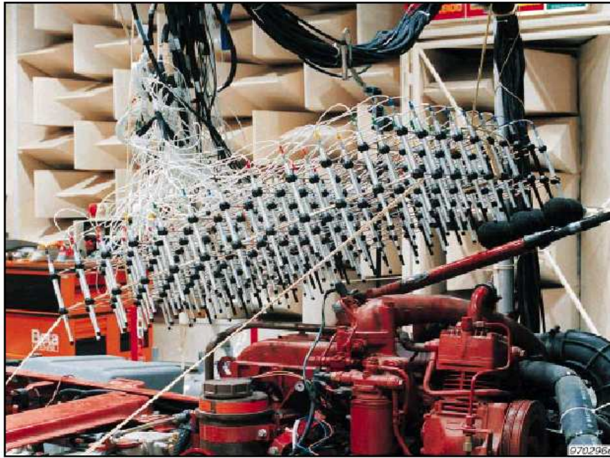
Figure 2.3: A typical engine test cell acoustic holography test setup with a planar microphone array.
